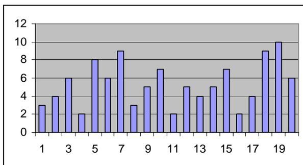
**Figure 4.** 20 faults and the number of activities in which they are properly recognized. Diagnosis performed on the target hydraulic system applied plausibility criteria from human diagnostician concerning patterns of manifestations-to-faults from practice and deep knowledge on specific transport anomalies for the faults in concern. Deep knowledge for
